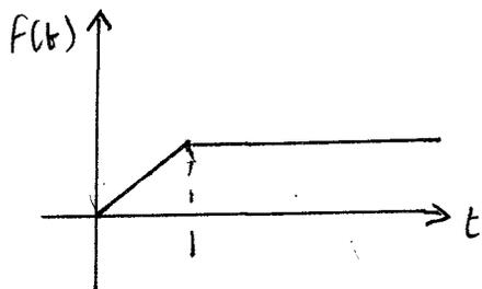
$$\begin{aligned} f(t) &= \begin{cases} t & 0 < t < 1 \\ 1 & t \geq 1 \end{cases} \\ &= t + \underbrace{(1-t) H(t-1)}_{\begin{cases} 0 & t < 1 \\ 1-t & t \geq 1 \end{cases}} \end{aligned}$$
