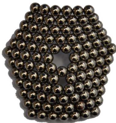
Fig. 9. A pentagon–heptagon pair in a hexagonal lattice
