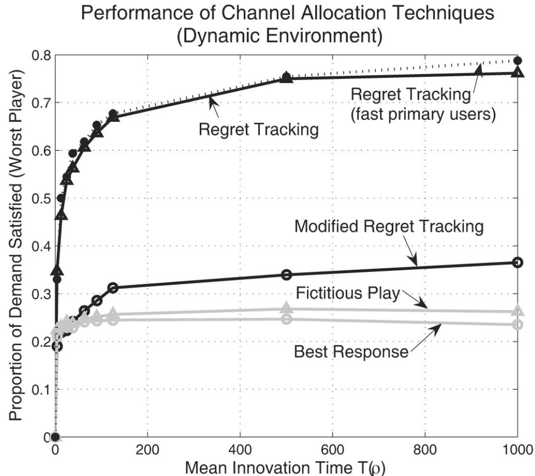
Fig. 6. Long-run average spectrum utilization in a dynamic environment for the channel allocation techniques of Section V.  $T(\rho)$  (see Sec.VI-C) is the mean time between innovations in the system (changes in primary user activity, fast primary user statistics or cognitive radio demands).
